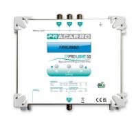
**3-input** (VHF+DAB / UHF flexible) **programmable head-end** to carry out high selectivity filters with up to  $108dB\mu V$  output level for each filter. **32 filters from 1 to 6 channels**, each with 9 selectivity levels.
